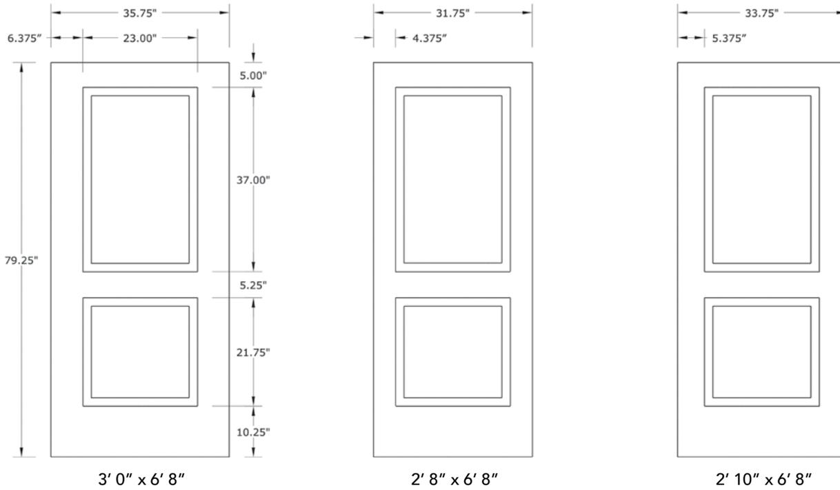
NOTE: BY REQUEST, DOOR HEIGHT COMES IN VARYING DIMENSIONS TO A MINIMUM OF 79". EXCESS WILL BE TAKEN FROM BOTTOM RAIL. ALL OTHER DIMENSIONS WILL REMAIN THE SAME.
